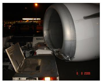
*Picture 1: The tug in contact with the engine (Source: AAS).*
