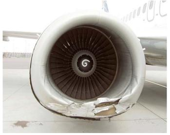
Picture 2: The damage to the engine nacelle.
