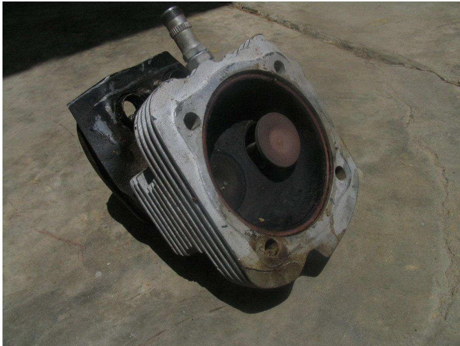
Figure 4. The exhaust valve stuck in an open position.
