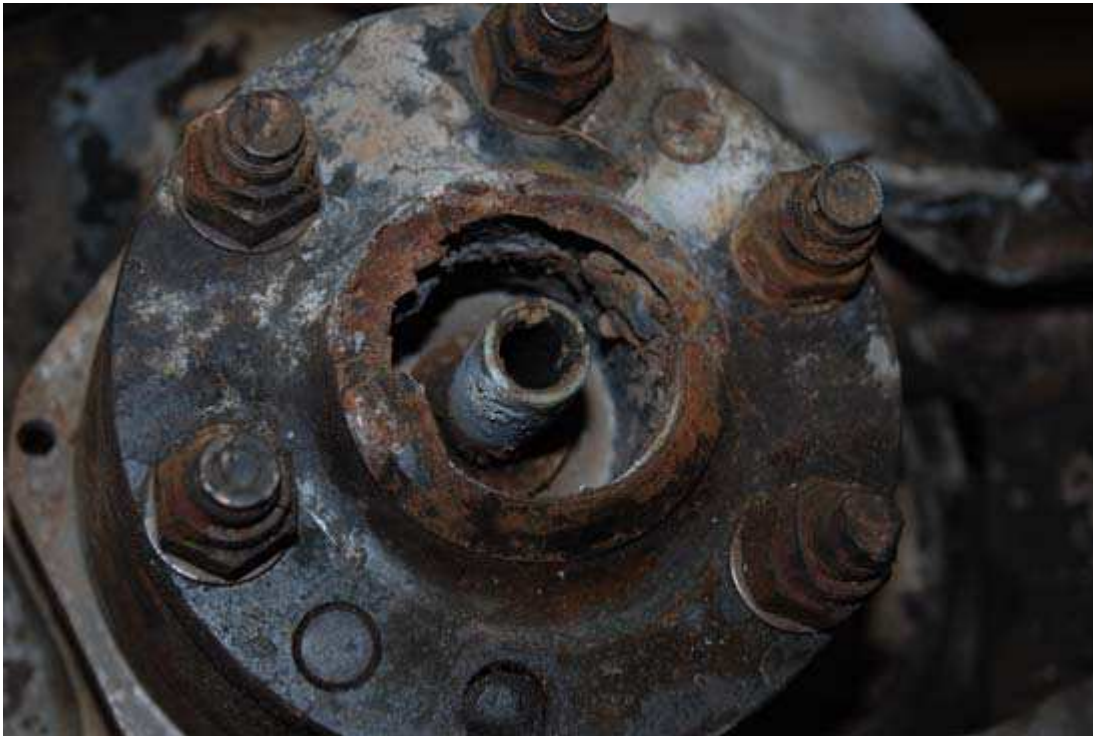
Figure 6: Damage to the propeller hub.
