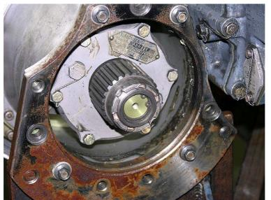
Figure 19 Main power drive spline in a serviceable condition
