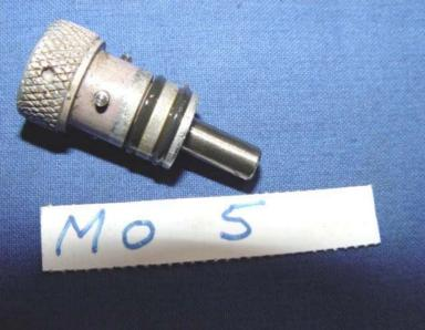
Figure 05 : Reduction gearbox (MO5) oil scavenge magnetic plug, free from metal particles
