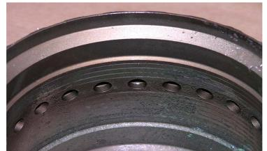
Figure 28 Turbine shaft labyrinth showing slight rubbing at the bottom plane
