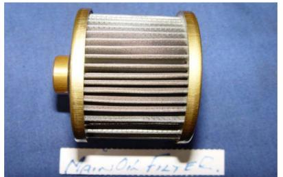
Figure 13: Engine main oil filter, contamination free.
