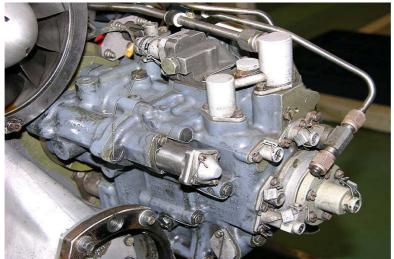
Figure 33: FCU showing the temperature compensator adjuster cover without the manufacturers Seal.
