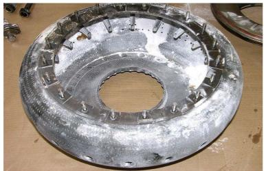
Figure 29: Combustion chamber
