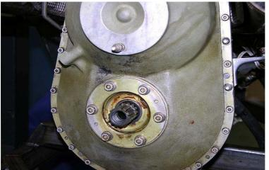
Figure 20 Tail rotor drive spline in a serviceable condition
