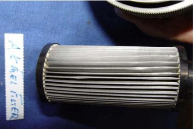
Figure 12: Aircraft fuel system filter, contamination free
