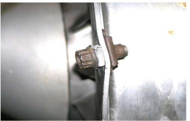
Figure 17 Axial compressor casing to air intake housing flange showing impact displacement
