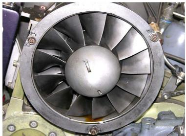
Figure 18 Axial compressor, no impact damage and erosion level satisfactory.
