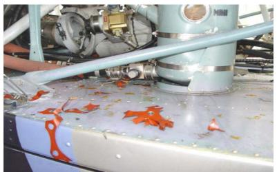
Figure 02 Flex coupling destruction
