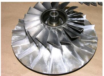
Figure 25: Centrifugal compressor showing fire extinguisher powder.
