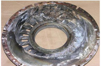
Figure 32: Axial compressor diffuser, contaminated, but free from operational anomalies.
