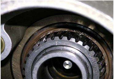
Figure 23: Drive gear securing nut rotational displacement of index marks
