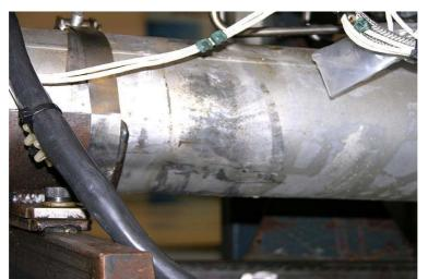
Figure 16 Impact damage to liaison tube
