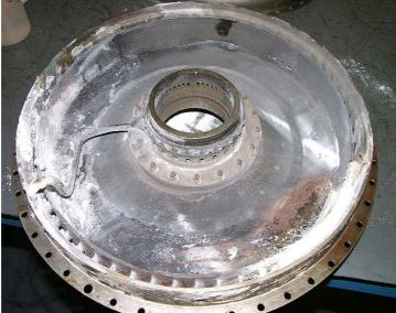
Figure 27: Centrifugal compressor diffuser and injection manifold assembly.
