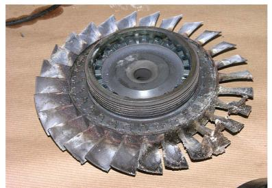
Figure 31: Gas generator turbine showing fire extinguisher powder contamination
