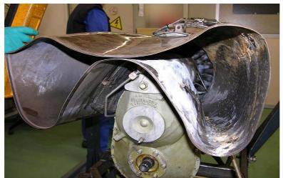
Figure 15: Impact damage to engine exhaust.
