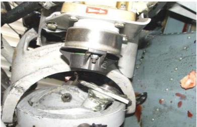
Figure 03: Main gearbox drive shaft impact ruptured disconnected.
