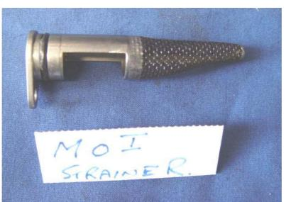
Figure 08: Accessory gearbox (MO1) oil return strainer, contamination free.
