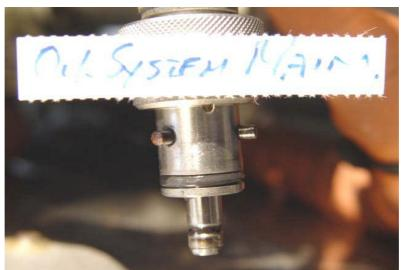
Figure 07 Oil system main chip detector, contamination free.
