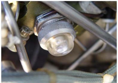
Figure 01: Main oil filter pre-blockage indicator not activated
