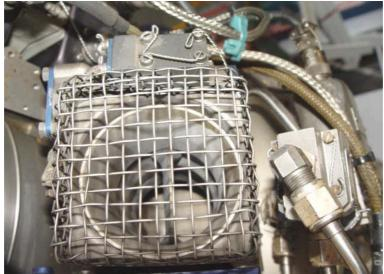
Figure 21: Compressor bleed valve in the open position.
