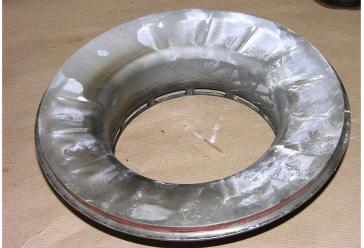
Figure 26: Centrifugal compressor casing showing slight rubbing
