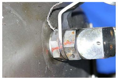
Figure 22: P3 air supply union to bleed valve
