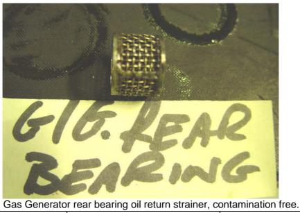
Figure 09:Gas Generator rear bearing oil return strainer, contamination free.CA 12-12a23 FEBRUARY 2006Page 24 of 32
