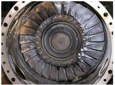
Figure 24: Power turbine contaminated with fire extinguisher powder
