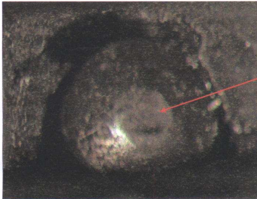
Photo 2: Failed piston guide pin position (stereo)
