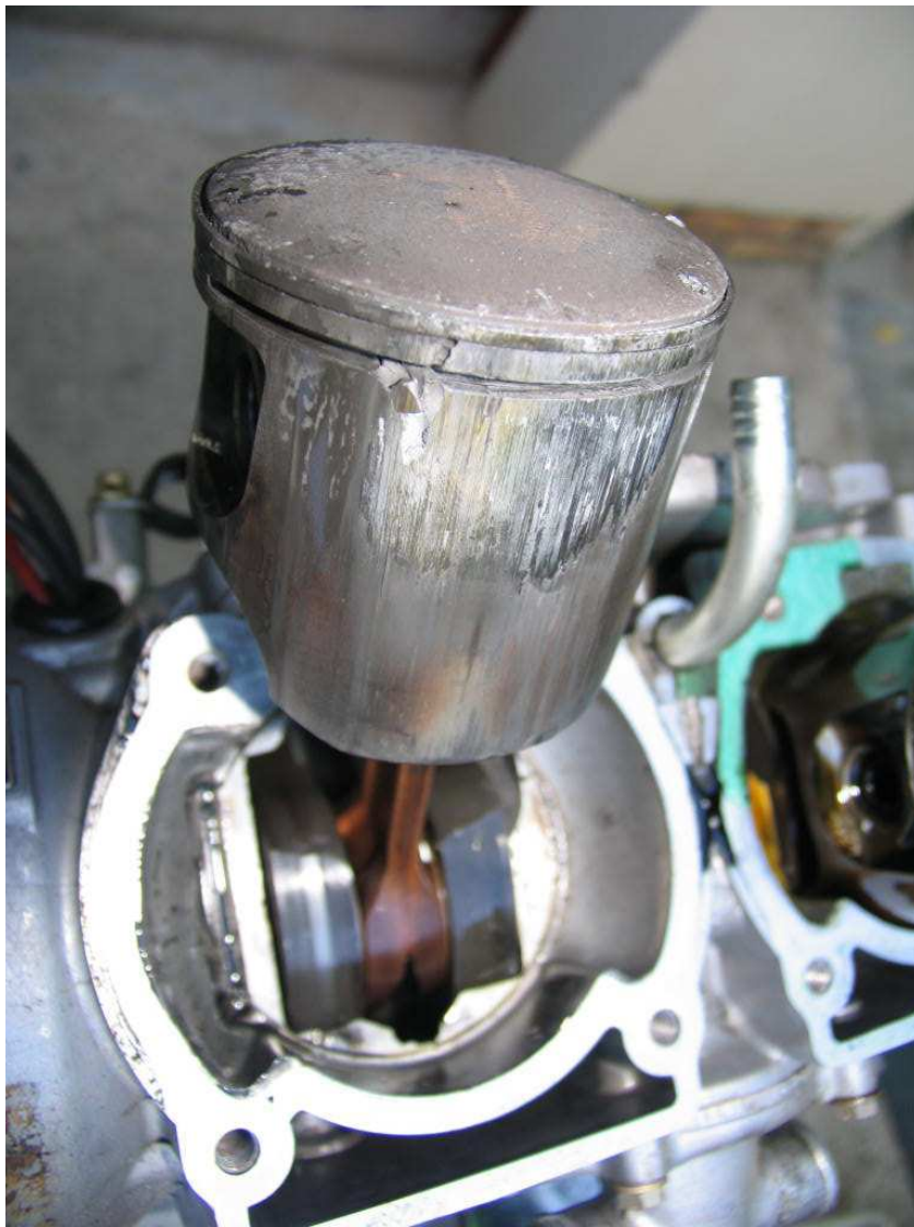
Figure 4. No. 2 piston displaying evidence of severe scuffing.
