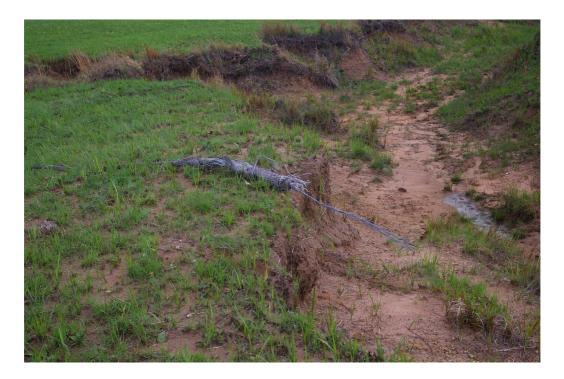
Photo 2 One end of the broken electrical cable on the ground.
