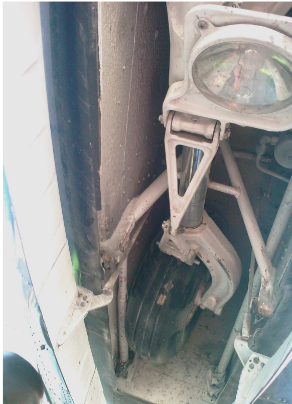
Figure 2. The nose wheel stuck in the wheel bay.
