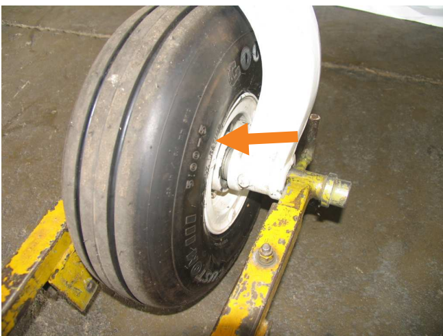
Figure 4. Two spacers on the right of the wheel.
