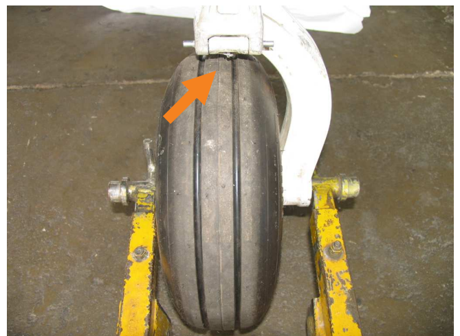
Figure 5. The wheel off-centre.
