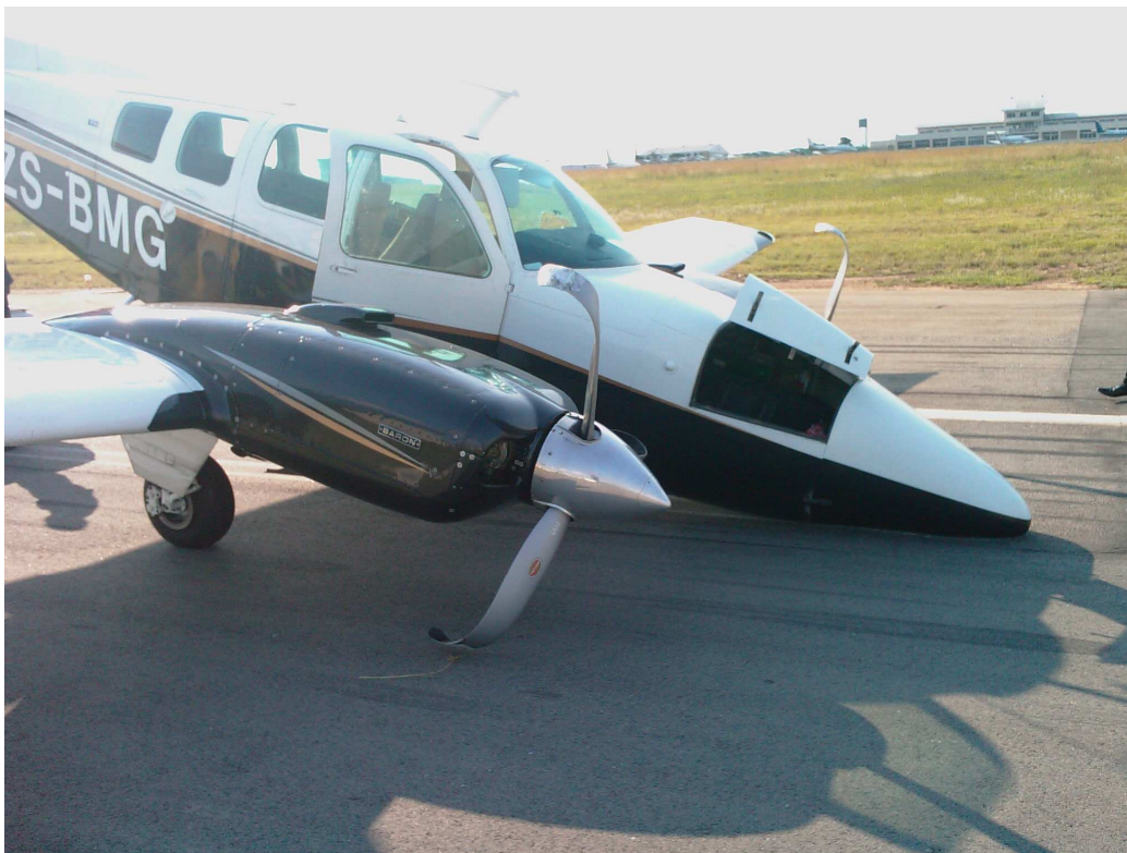
Figure 1. The aircraft after the landing with its nose wheel in a retracted position.
