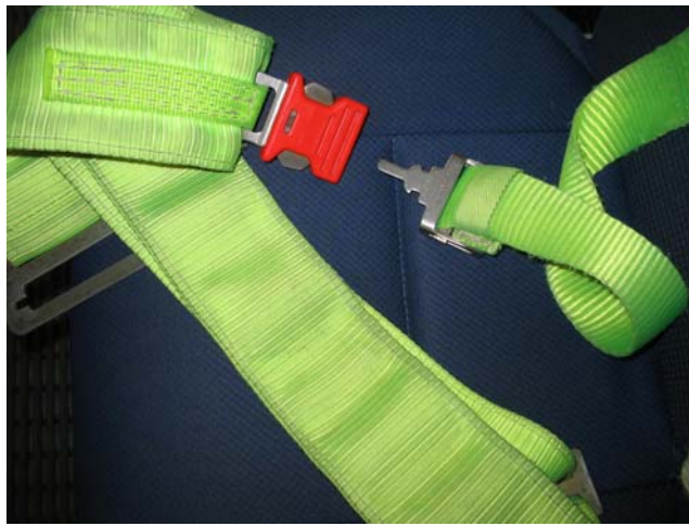
Figure 11: A view of a “monkey chain/belt” waste area, plus a safety latch with quick release mechanism.
