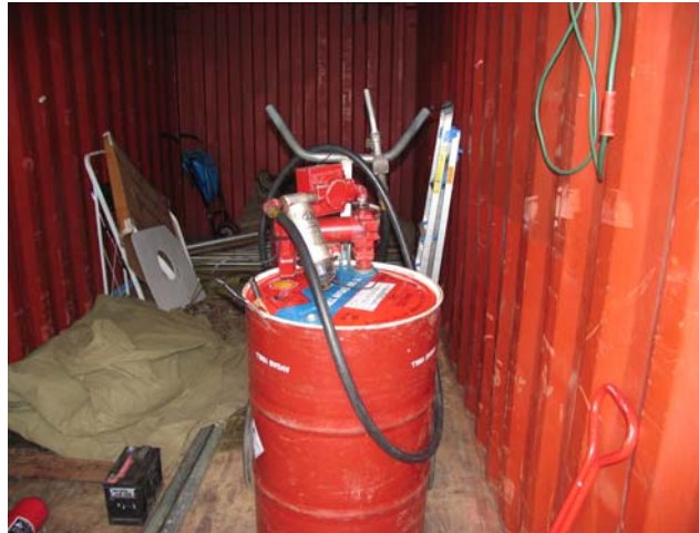
Figure 7: Indicating the drum from which the aircraft was refueled and way it was stored..
