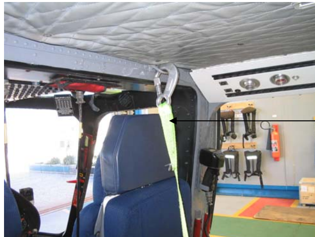
Figure 10: A view/illustration of a “monkey chain/belt” being secured to the roof structure of an aircraft.
