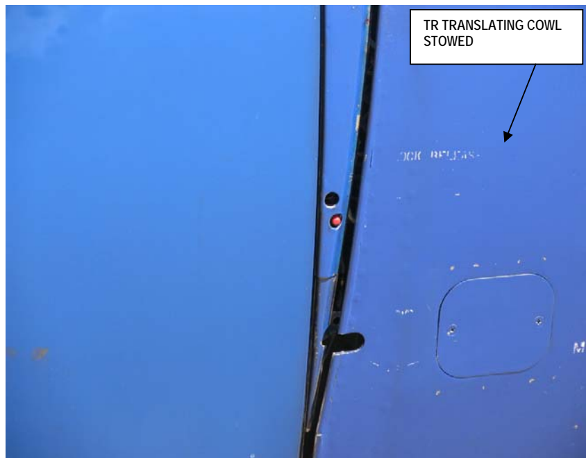
PHOTO 7: SHOWS THE TRANSLATING COWL IN THE FWD STOWED POSITION.
