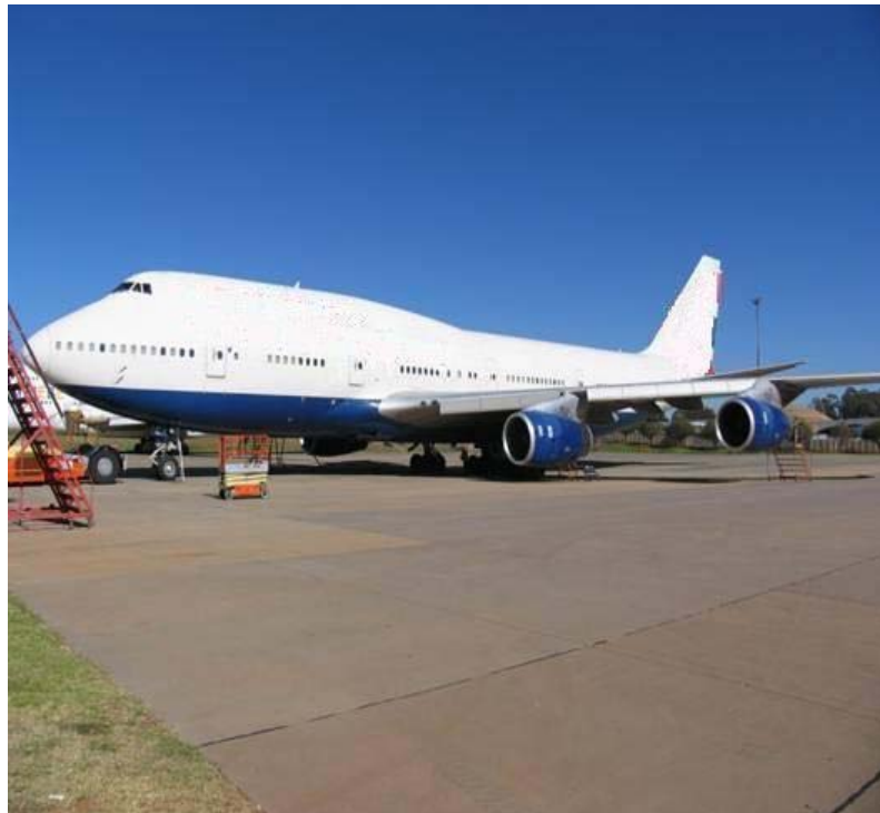
VIEW OF THE B747-400 G-BYGA WITH GROUP 'A' LEADING EDGE FLAPS EXTENDED ON THE LEFT HAND WING (RIGHT HAND WING LE FLAP CONFIGURATION IS SIMILAR).
