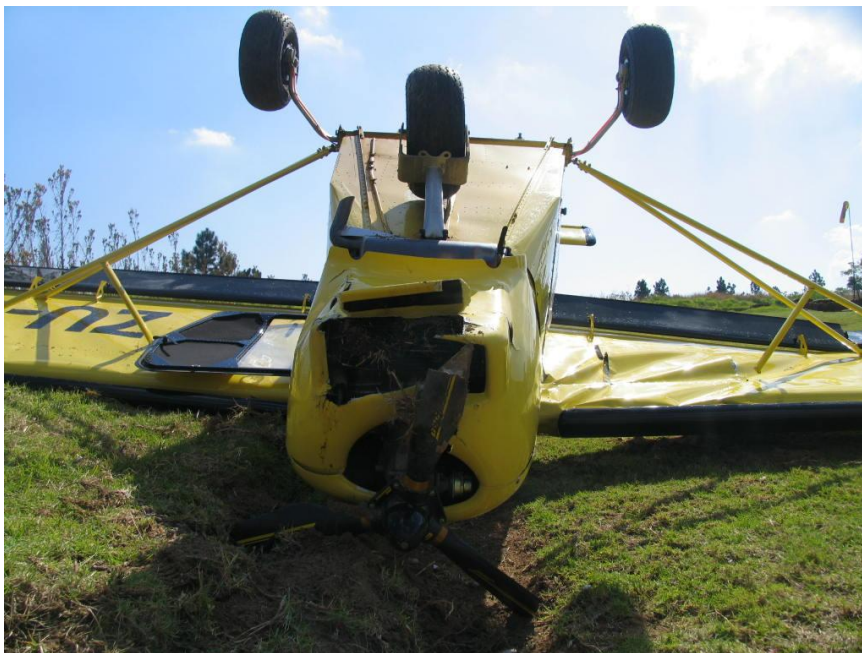
Photo 1: Broken propeller, collapsed nose gear and damaged wings
