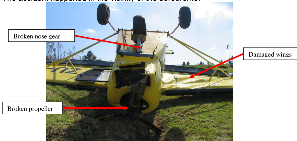
Photo 2: Showing damage to the aircraft
