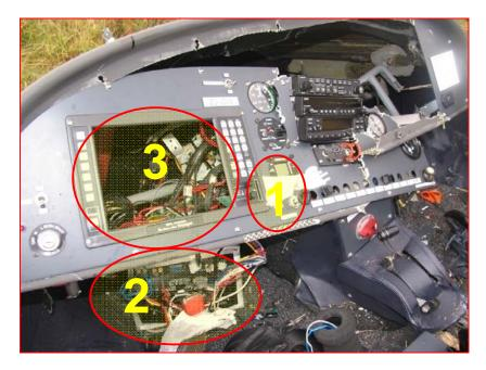
Figure 5: Circle 1 indicates the slot for the memory card. Circle 2 indicates the position of the EFIS after the accident and circle 3 the normal position of fitment for the EFIS.
