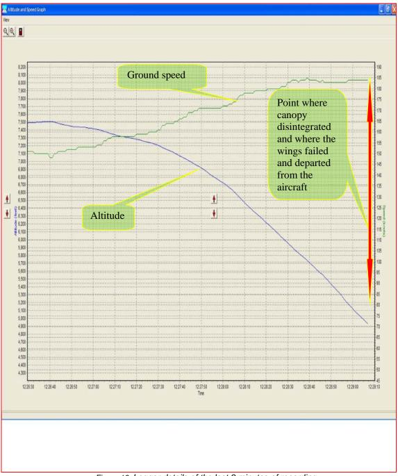
Figure 16: Logger details of the last 3 minutes of recording
