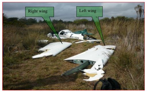
Figure 11: LH & R/H wing after recovery
