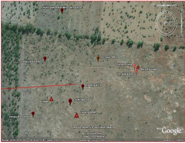
Figure 7: Wreckage distribution on accident site reference: Google Earth
