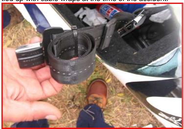
Figure 13: Both shoulder harnesses were tied up with cable ties, i.e. not worn
