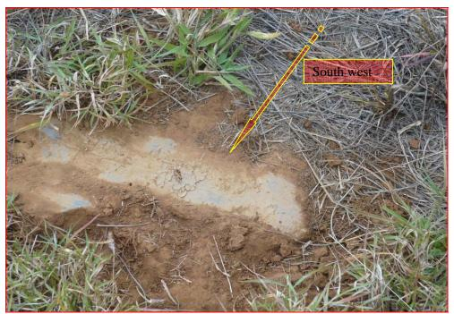
Figure 12: Initial impact point of the fuselage with the arrow indicating the direction of movement
