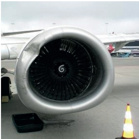
Illustration 4: damaged left engine cowling
