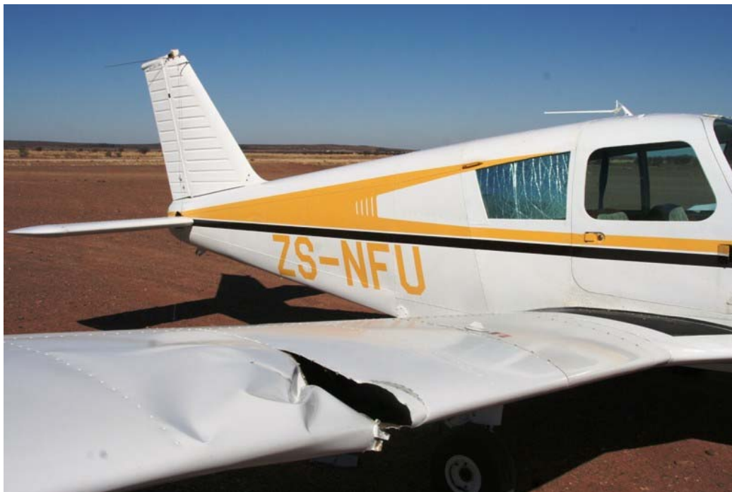
Figure 1. Damage to the wing.
