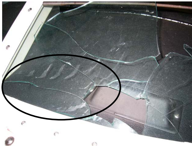
Figure 4. Marks on the broken (left) windshield similar to marks on the right windshield.
