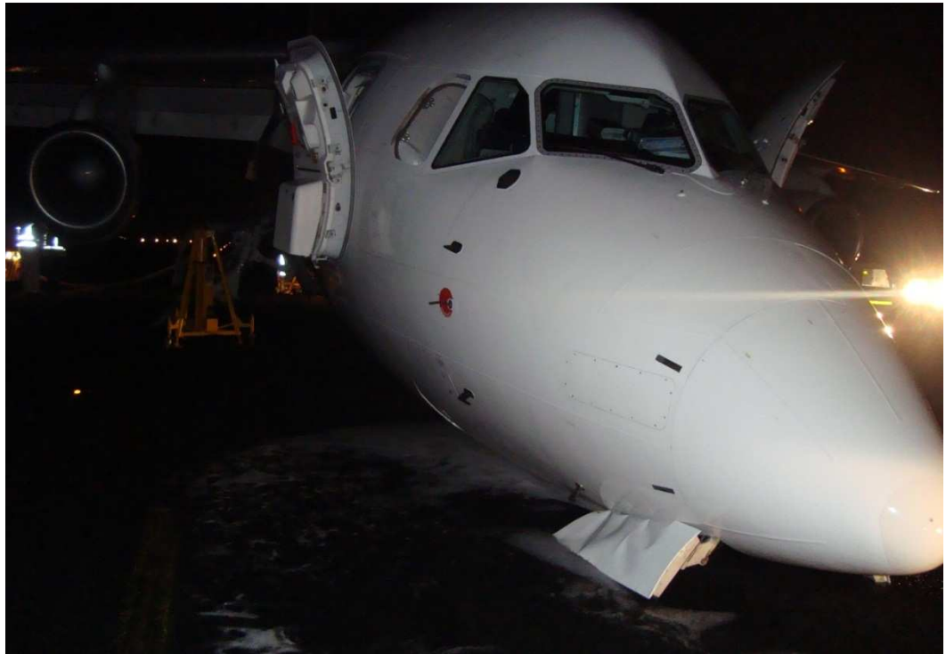
Figure 1, shows the BAE 146-RJ85 aircraft on the runway with the nose landing gear in the retracted position.
