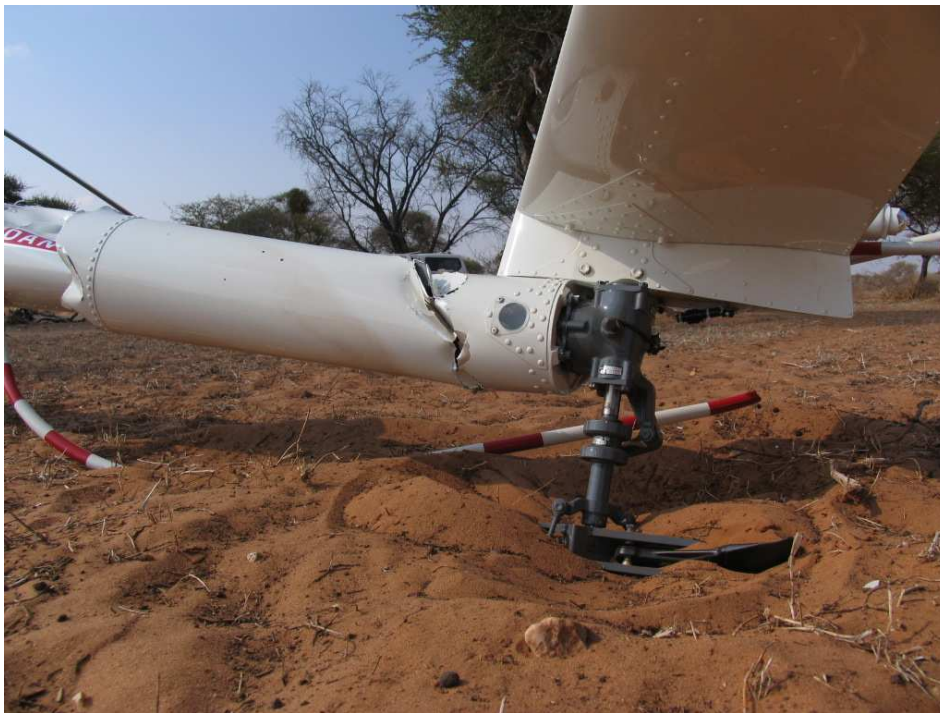
Figure 4. A view of the tail rotor assembly with rotational evidence visible in the sand.
