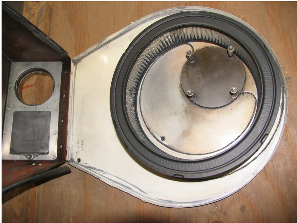
Figure 12. A view of the air filter box in the open position with the air filter and alternate air door visible.
