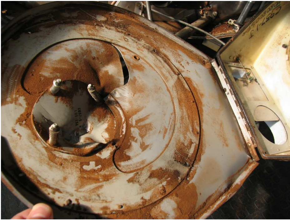
Figure 7. A view of the inside of the air filter box.
