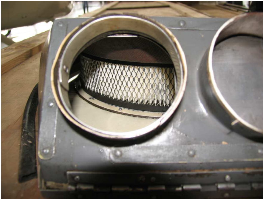
Figure 13. A view of the air box close with the air filter visible in position.
