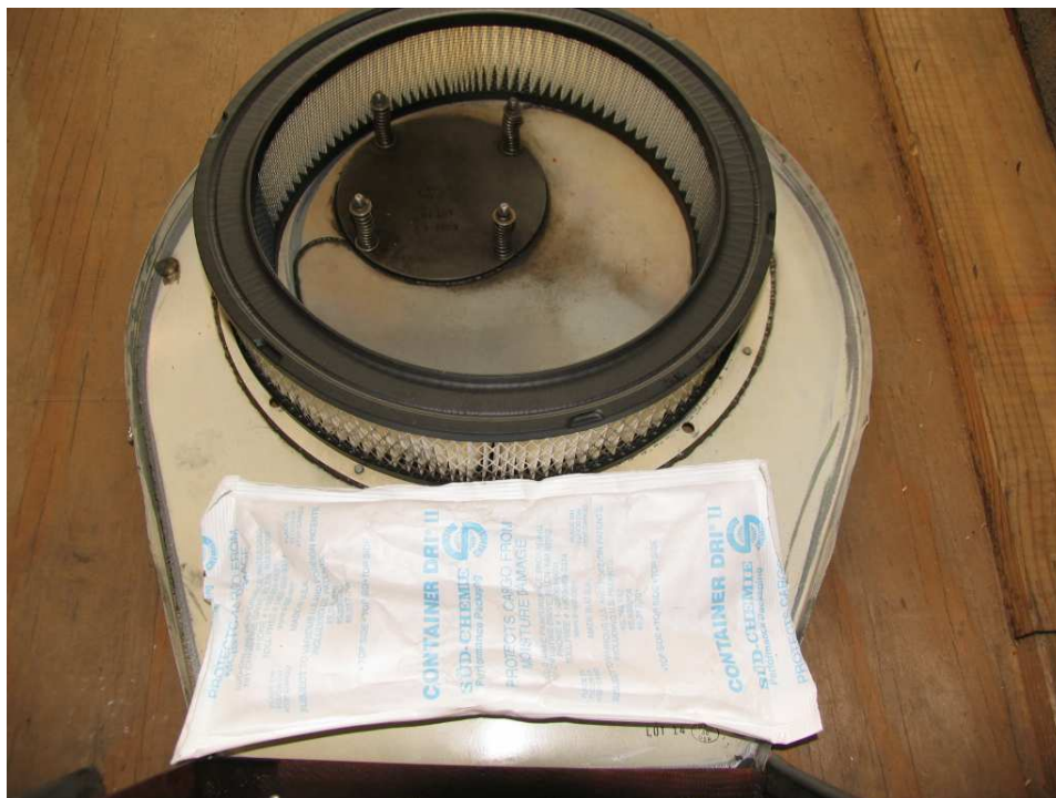
Figure 18. Moisture absorbent bag within the air filter box (for illustration purposes only).
