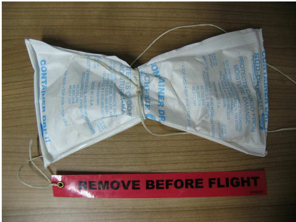
Figure 10. Moisture absorbent bag with the warning label attached used during shipment of a new helicopter.
