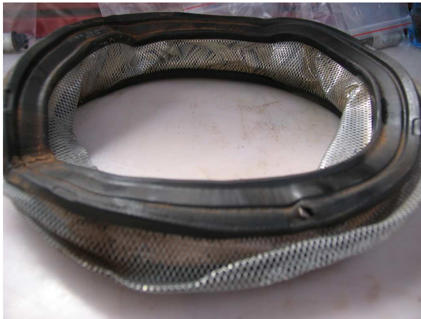
Figure 9. A view of the air filter that was in the filter box at the time of the accident.
