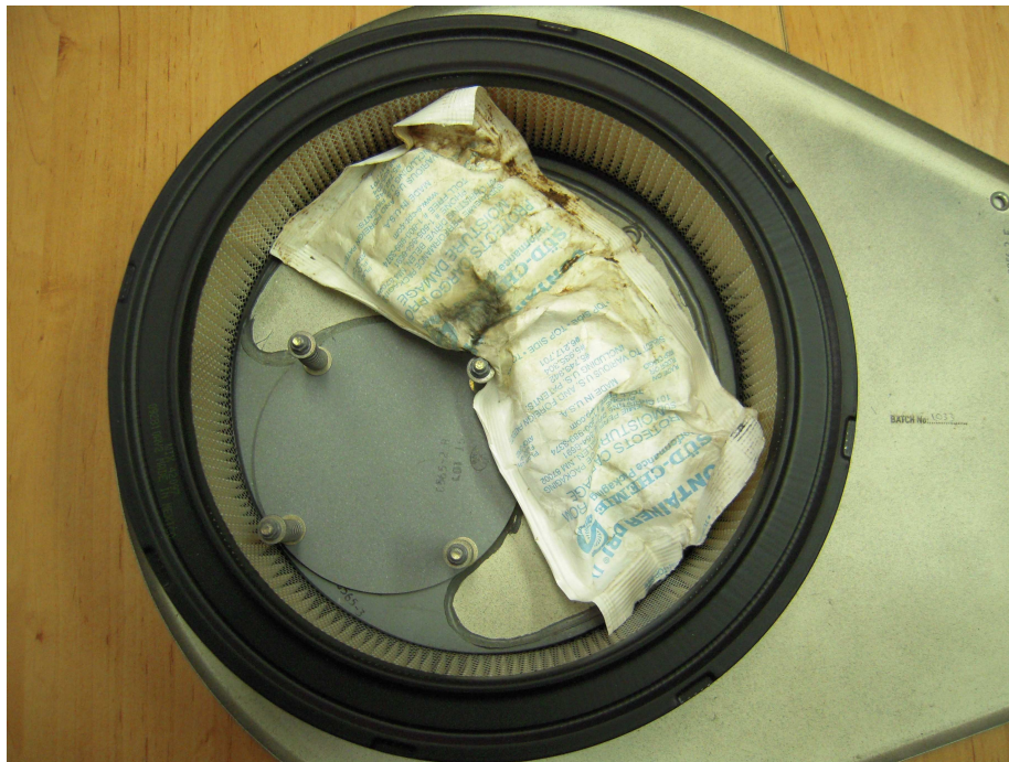
Figure 17. Moisture absorbent bag within the centre of the air filter box (for illustration purposes only).
