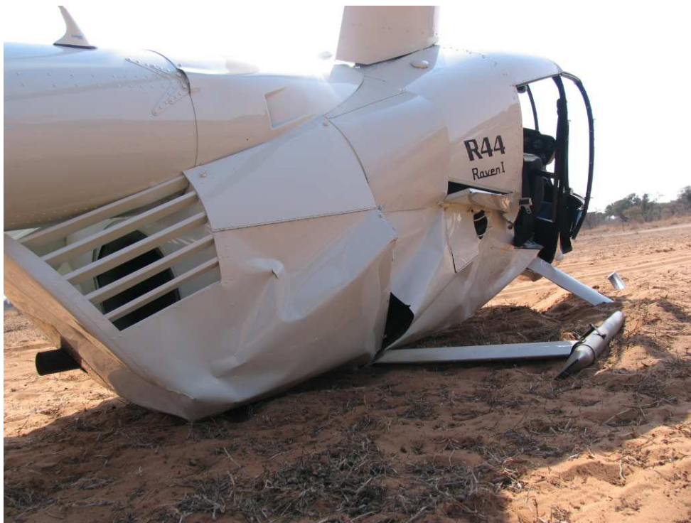
Figure 2. A view from the right aft position with the right aft skid gear flattened.
