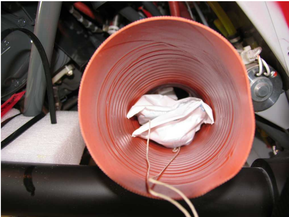
Figure 15. The two moisture absorber bags visible inside the air inlet hose (ropes to the warning labels).
