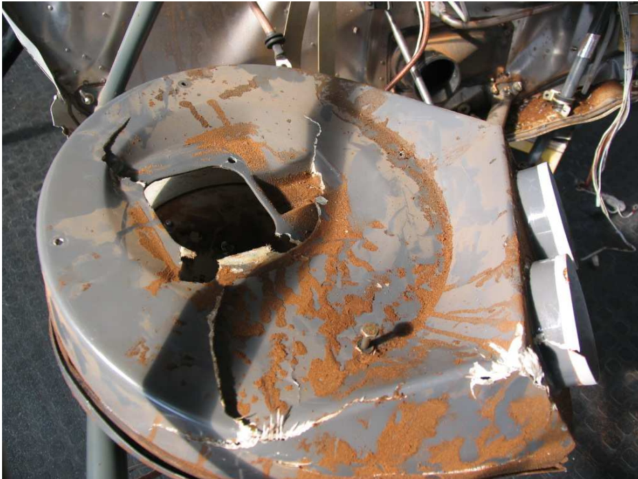
Figure 8. A view of the top of the air filter box where the carburettor gets attached to.
