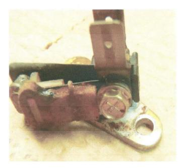
Picture No.1 - Corrosion on Points Assembly Bracket - Right Magneto
