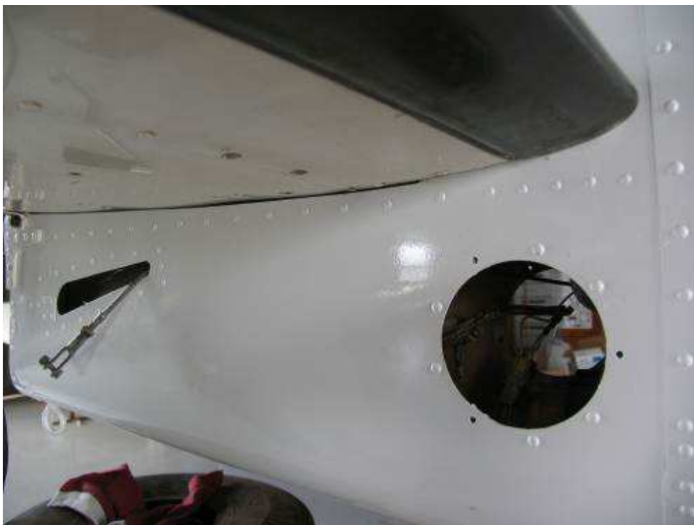
Figure 7. On the photo the inspection panel is removed and the rudder cable disconnected (maintenance)
