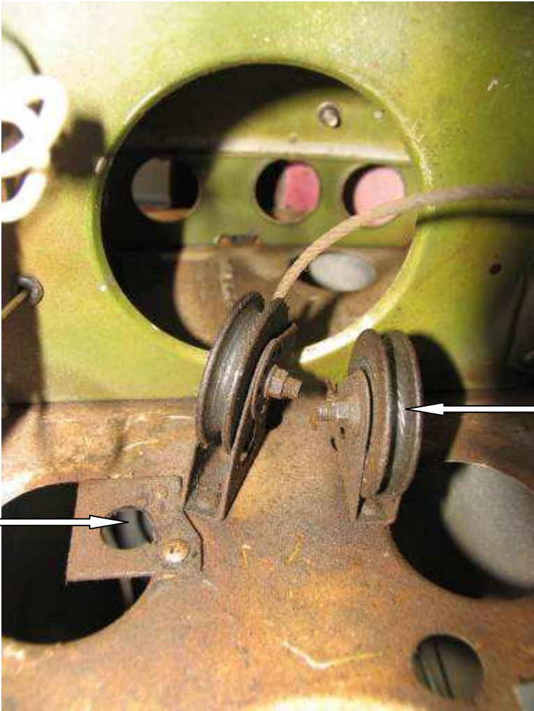
Figure 10. A close-up view of the pulley (Section A) that supports the right-hand rudder cable
