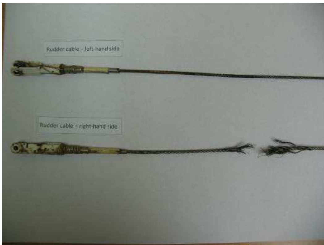
Figure 16. A view of the aft section of the two rudder cables.
