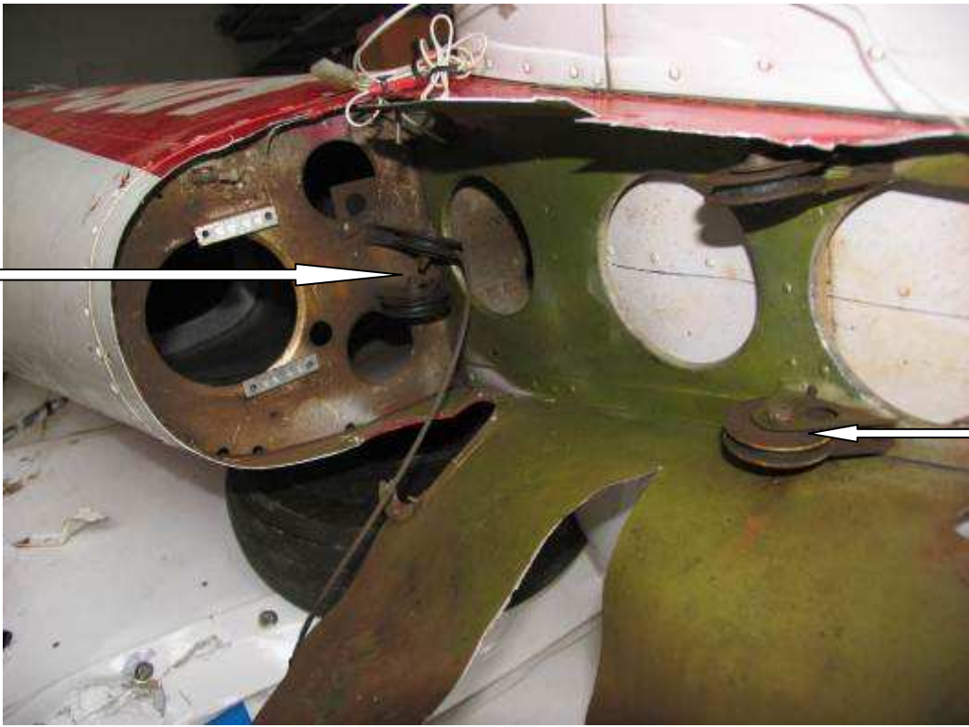
Figure 9. The aft section of the fuselage cut open in order to inspect the rudder cable pulleys
