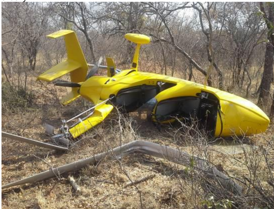
Figure 2: The autogyro fell over onto its right side after striking the trees.
