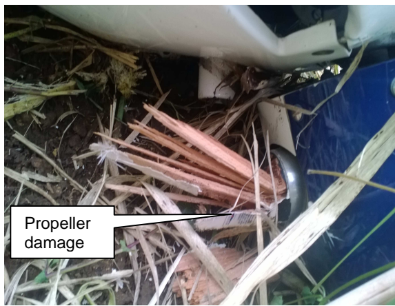
Figure 6: Shows propeller damage
