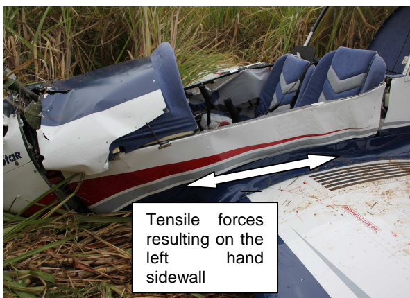
Figure 3: Left hand side view of the damage
