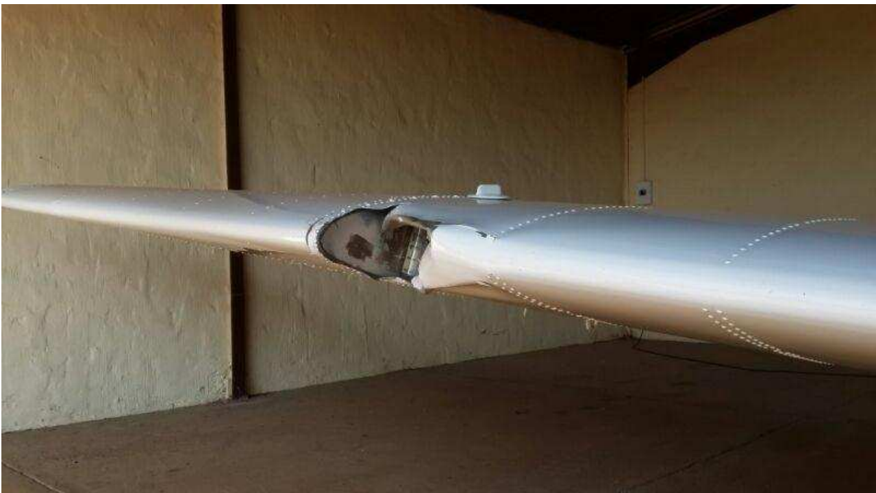
Figure 1: The damage to the right wing of ZS-MEA after impact.
