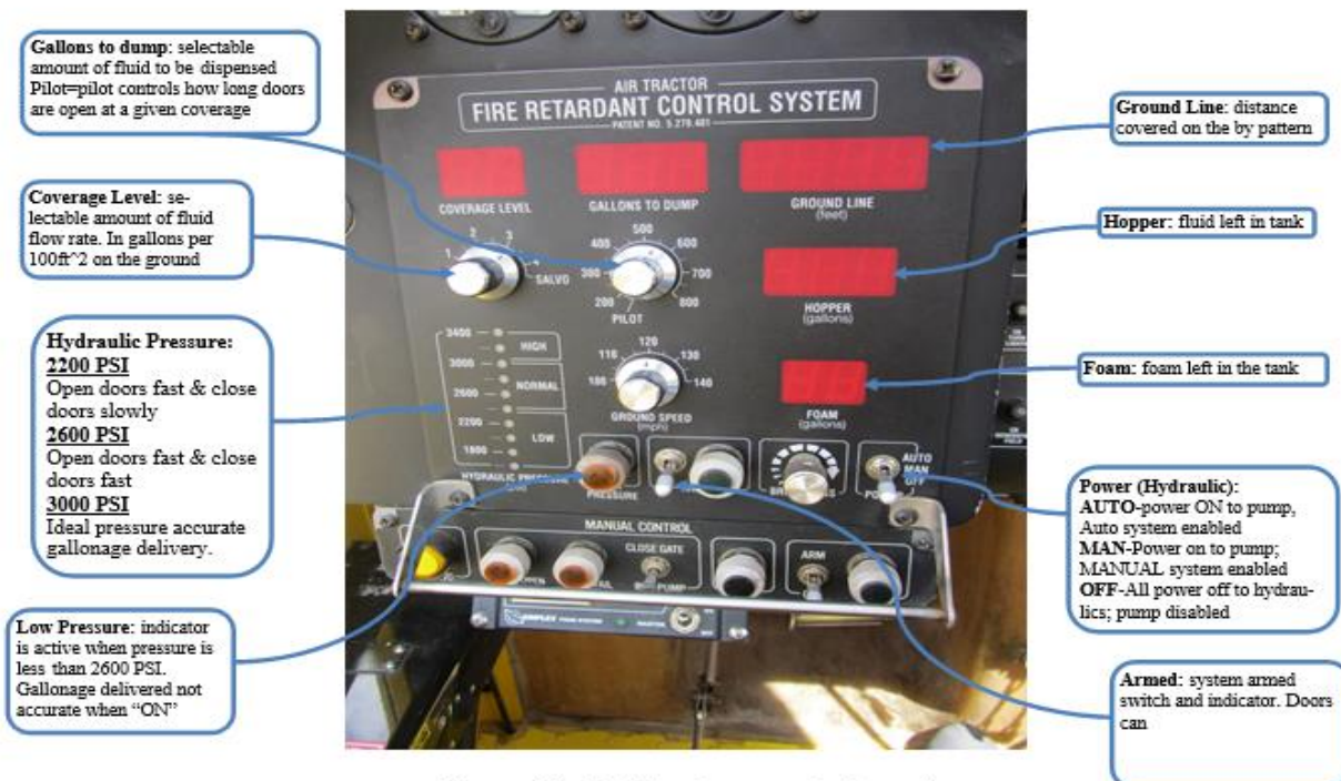
Figure 12: FRDS primary control panel
