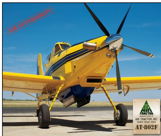
Figure 7: showing gatebox doors in an open position (Courtesy of Air Tractor website)
