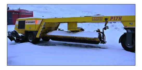
The snow clearing width of each snow clearing sweeper was 4 meters.
