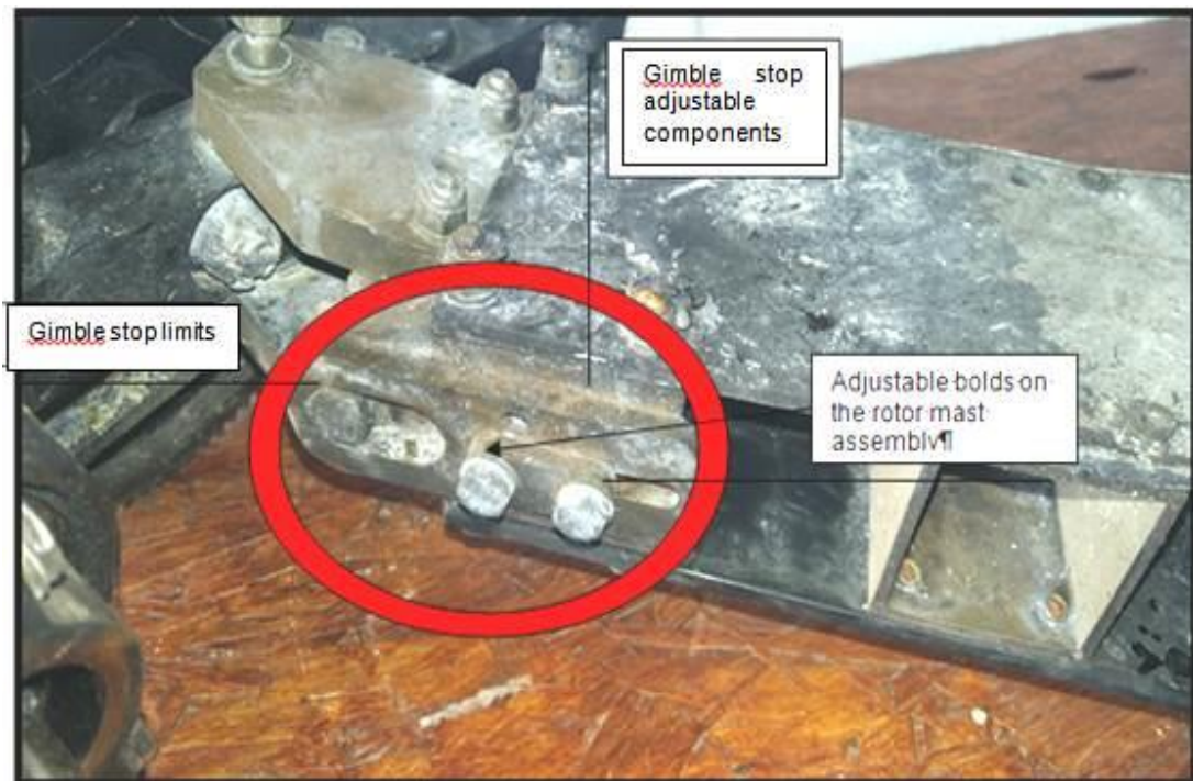
Figure 11: Shows the mast assembly gimble head/stop adjustment as found on the accident aircraft
