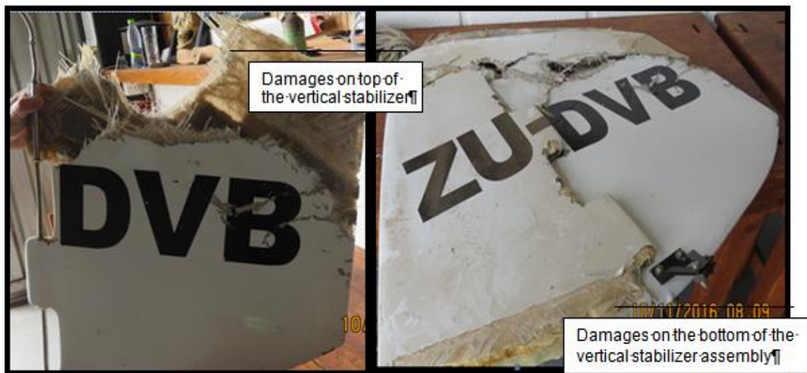
Figure 7: Shows the damages on the vertical stabiliser
