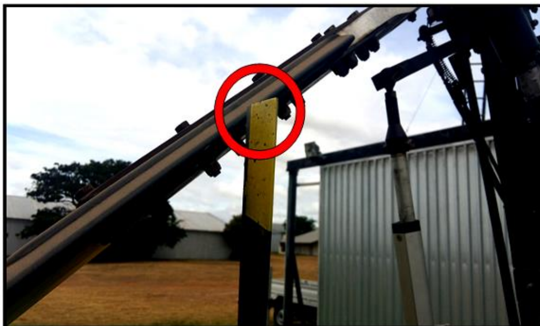
Figure 10: Contact possible when bolts are set to the position as they were found on the accident aircraft
