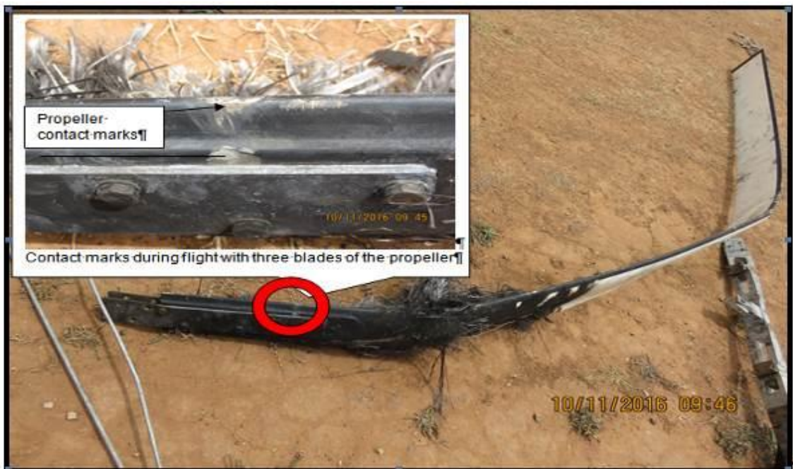
Figure 6: Shows damage to the rotor blade and the contact mark with the propeller blades
