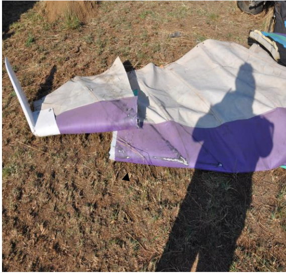
Figures 12: Failed rightwing displaying witness marks sustained after the collision
