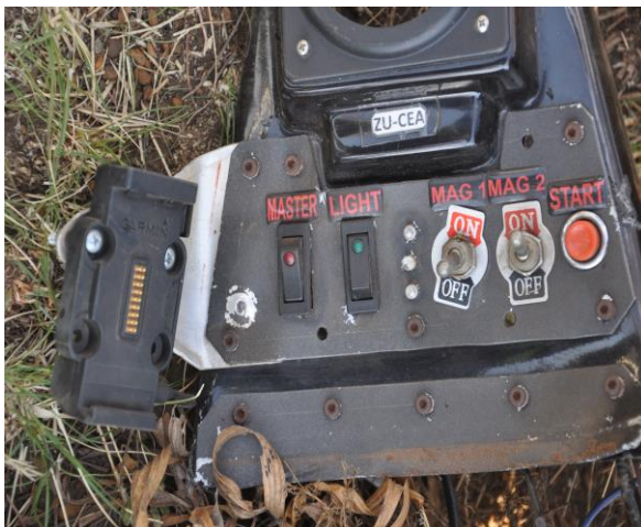
Figures 14: The aircraft dash showing the master with the magneto switches and the main landing gear with no fairings fitted to them
