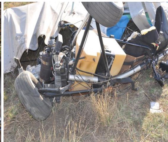
Figures 14: The aircraft dash showing the master with the magneto switches and the main landing gear with no fairings fitted to them
