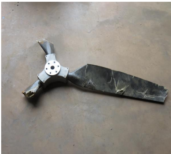
Figures 13: Accident severed propeller blades and the engine after they were separated
