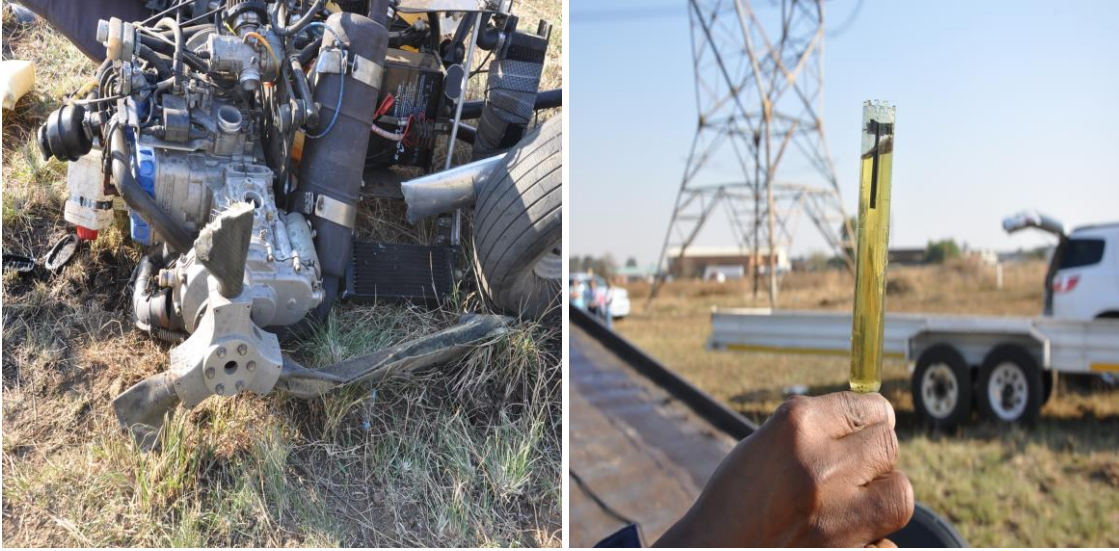
Figures 15: Accident severed propeller blades and the fuel sample taken during the on-site investigation
