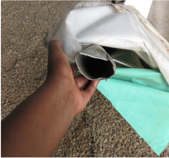
Figures 12: Failed rightwing displaying witness marks sustained after the collision
