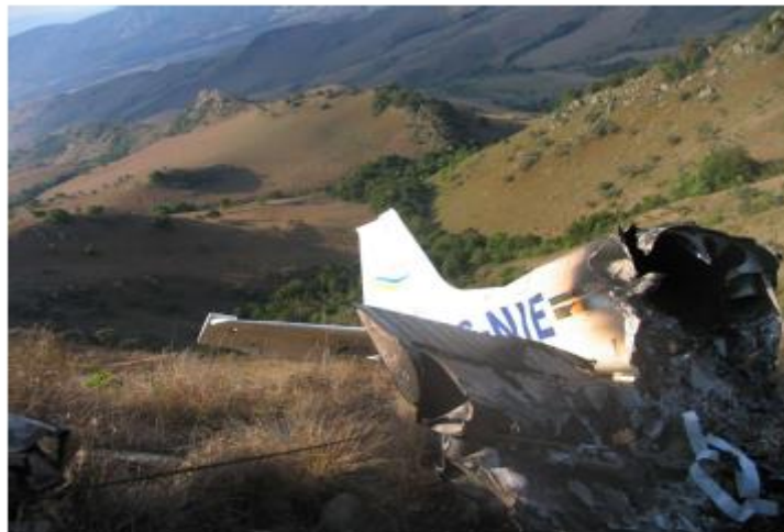
The aircraft collided with mountainous terrain during Instrument Meteorological Conditions (IMC) on a flight from Nelspruit Aerodrome to Rand Aerodrome.
