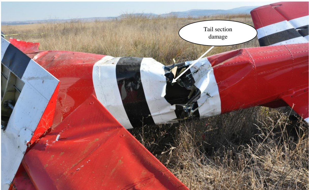
Figure 6: Tail section showing compression damage
