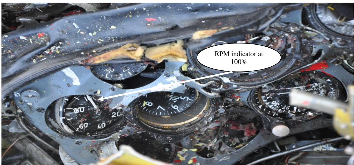
Figure 3: Showing the RPM indicator at 100%
