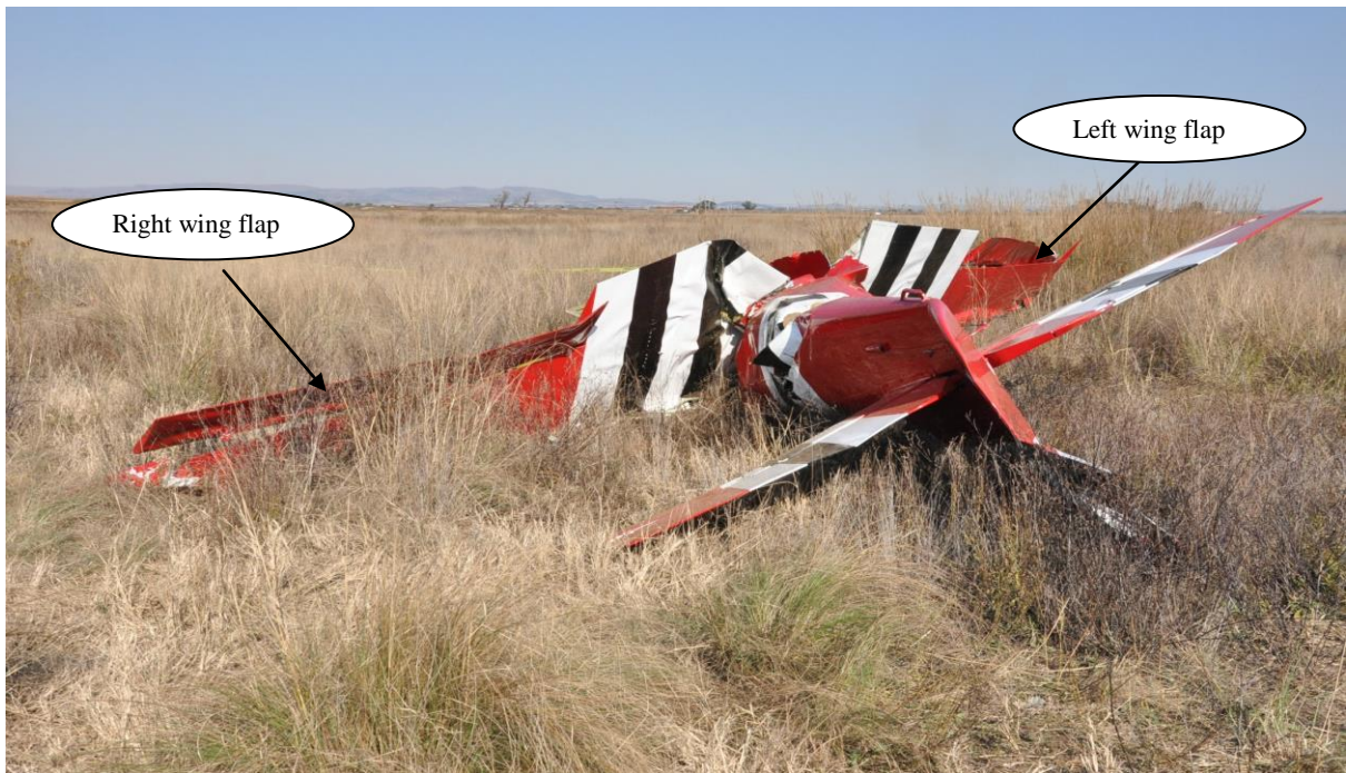
Figure 7: Showing damage and the position of the wing flaps
