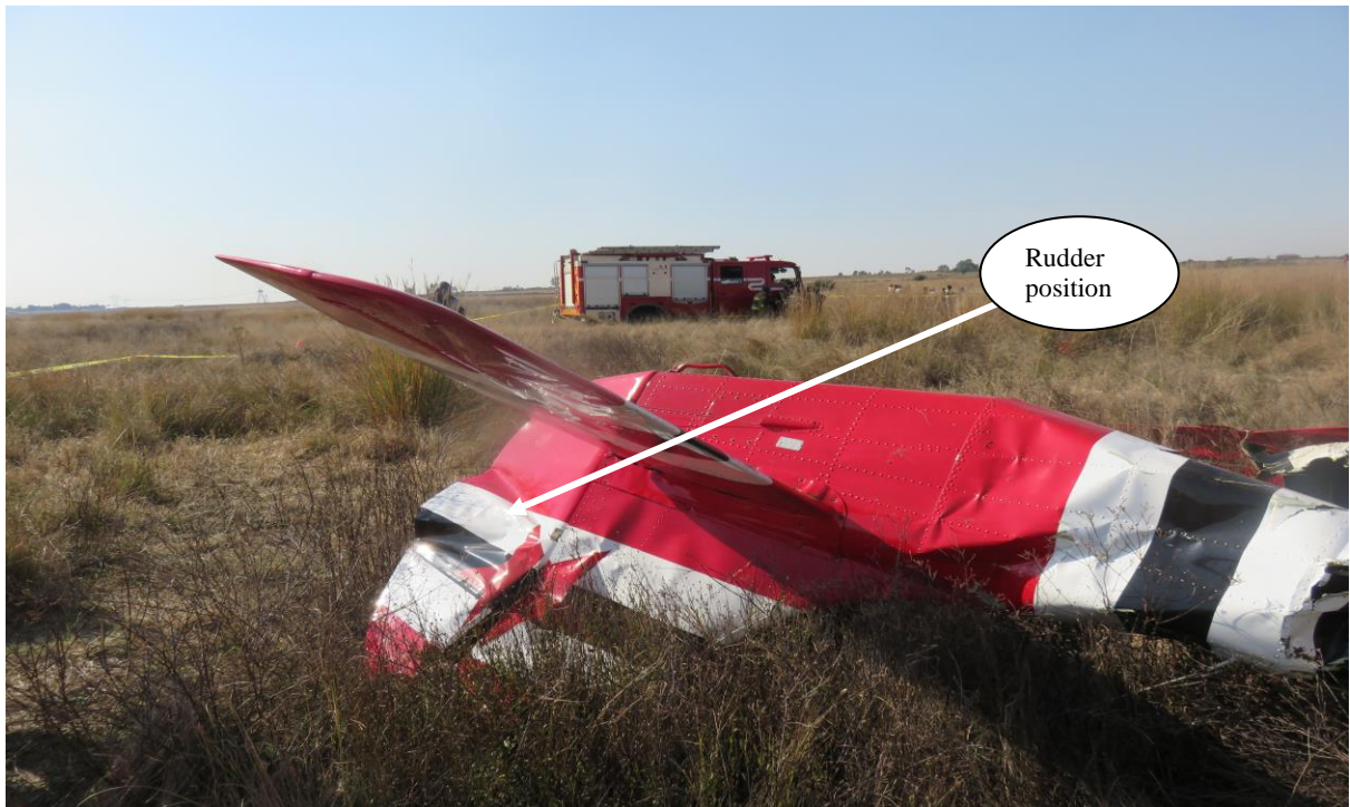
Figure 5: Arrow showing the rudder position as found after impact with the ground
