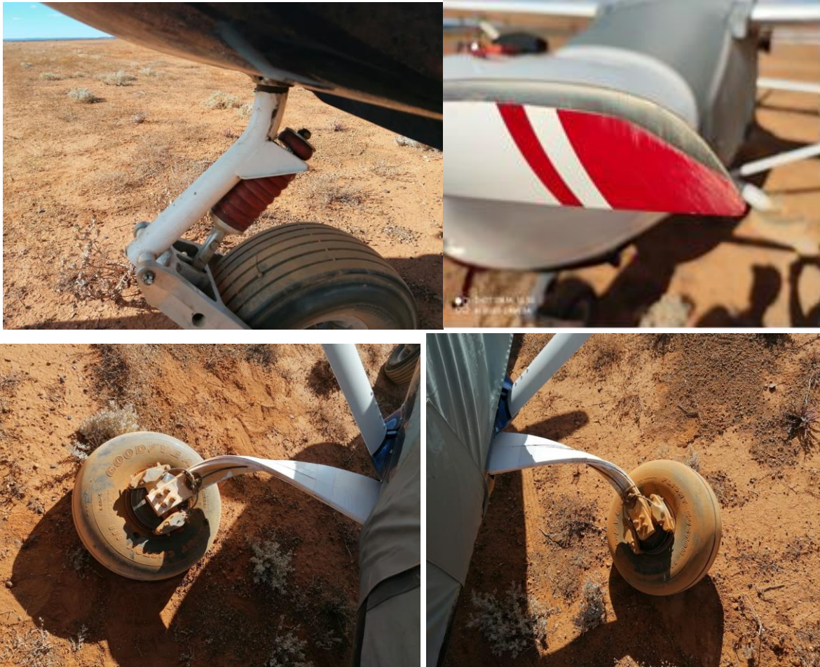
Figures 1, 2, 3 & 4: Damage to the nose gear strut (top left), one of the propeller blades (top right), left main landing gear (bottom left), and right main landing gear (bottom right). Damages are all consistent with hard landing.
