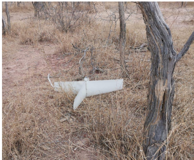
Figure 2: The helicopter's severed stabiliser. (Source: Pilot)
